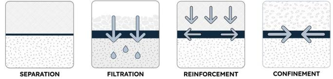
MIRAFI® HP370 geotextile is composed of high-tenacity monofilament polypropylene yarns, which are woven into a network such that the yarns retain their relative position. MIRAFI HP370 geotextile is inert to biological degradation and resistant to naturally encountered chemicals, alkalis, and acids.
