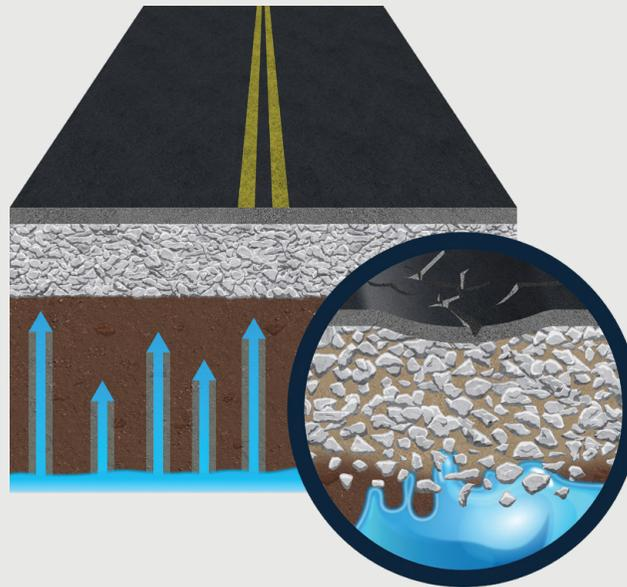
As capillary action causes groundwater to rise into the stress zone underneath the road, the strength of the road decreases, leading to damage over time.
