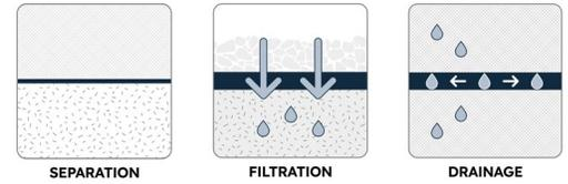
MIRAFI® E1200 is a needlepunched nonwoven geotextile composed of polypropylene fibers, which are formed into a stable network such that the fibers retain their relative position. MIRAFI E1200 is inert to biological degradation and resists naturally encountered chemicals, alkalis, and acids.
