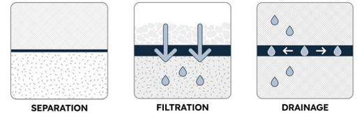
MIRAFI® 1100NC is a needlepunched nonwoven geotextile composed of polypropylene fibers, which are formed into a stable network such that the fibers retain their relative position. MIRAFI 1100NC is inert to biological degradation and resists naturally encountered chemicals, alkalis, and acids.
